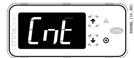
3. Press PRG to activate the continuous cycle (Cnt). Press DOWN to activate the next function;
