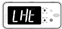
2. Press PRG: Lht is displayed, the UP and DOWN buttons light up. Press PRG to turn the light on/off: the icon will come on or go off. Press DOWN to activate the next function (Cnt) or press Esc to exit;
